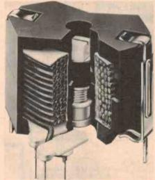
Cutaway view of a potcore showing the winding on the internal bobbin and the inductance adjustor in the centre. The ferrite 'pot' comes in two halves, held together with a clip.
