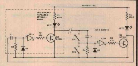
lower threshold. When it does, the output of IC1b will go low and Q2 will turn off. Then, C1 will charge via R6 and LED2, but the initial pulse will turn Q1 on via IC1a and LED1 will light. When C1 charges such that the input of IC1a goes below its lower threshold, Q1 will turn off, triggering the next inverter stage in the chain and so on, right
