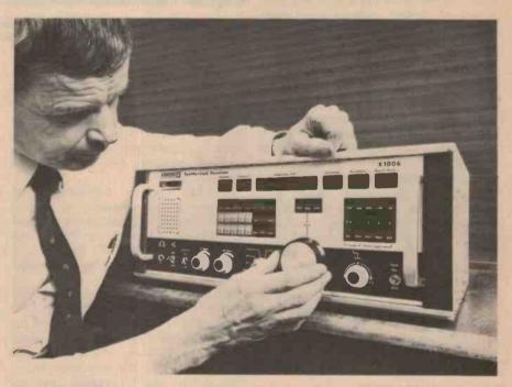
The Redifon R1006 receiver can control up to 99 remote receivers over any distance by ordinary telephone lines or radio links as appropriate.
