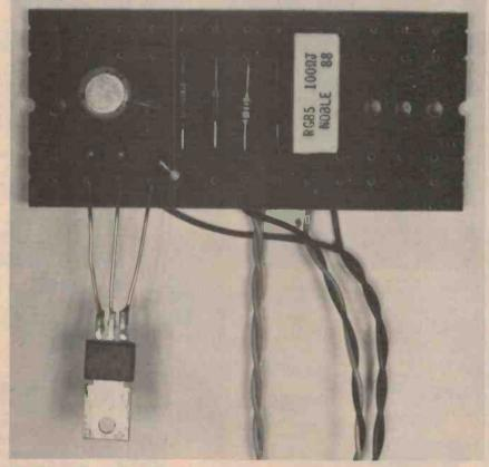
Showing the components mounted on the tagstrip.
