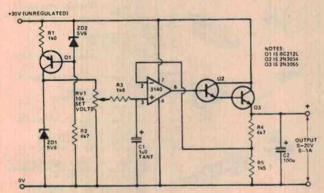
Figure 5. This circuit is a little more sophisticated and performs better than the Figure 4 circuit. This circuit will deliver up to 1 A output current, output voltage being variable between 5.6 V and 15 V. Thermal drift is near zero.
