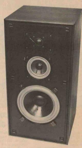
the on-axis response and the general frequency response characteristics are above average. The individual responses of the three drivers have been very well selected and the crossover frequencies are well chosen. This is borne out by the phase response of the unit, which is exceptionally flat and shows how effective the design is in reducing phase differences.
