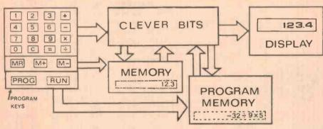
Figure 3 shows a simplified block diagram of a programmable calculator. By now we're getting close to a computer.
