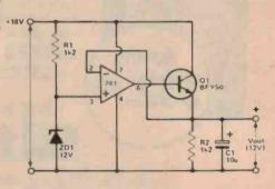
Figure 4. A considerable improvement in regulation is achieved by employing a high gain op-amp to drive the series pass transistor plus negative feedback from the dc output. This circuit will deliver up to about 100 mA and the output voltage stays within a few millivolts of the zener reference for output current variation from zero to maximum.
