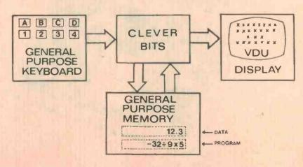
Figure 4. A computer has one large and versatile memory for both program and data.
