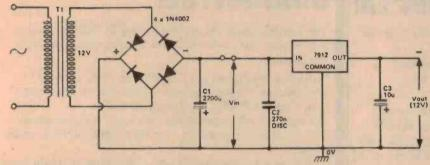
Figure 9. The negative voltage rall counterpart of Figure 8. Don't forget heatsinks.
