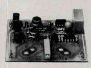
The meters comprise a sophisticated meter movement with fast ballistics and an amplifier with a high input impedance and low thermal drift. More information from the distributors, R.H. Cunningham Pty Ltd at P.O. Box 4533, Melbourne, Vic. 3001. (03) 329-9633 or P.O. Box 214, Neutral Bay Junction, NSW 2089. (02) 909-2388.
