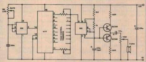
of the audio oscillator is fed to a complementary pair of transistors which drive a speaker for the audio output.
