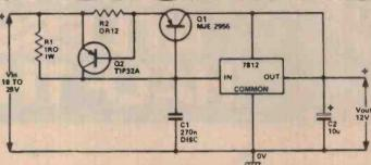
Figure 14. Adding current overload protection to the Figure 13 circuit. It's a wise idea, even though three-terminal regulators generally incorporate thermal shutdown protection.
