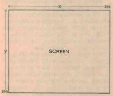
Figure 1. Pixels are addressed with x and y coordinates.
