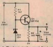
Figure 3. The basic 'serles pass' fixed voltage regulator using a zener reference. This circuit can deliver up to about 100 mA at 11.4 volts. Q1 is basically an emitter follower, the base being 'clamped' at 12 V by the zener. C1 reduces the circuit's ac impedance.
